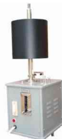
Cat No. 806(64) Kymograph Drum Electrical
